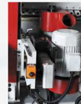
立轴系统 Moulding unit 5HP (special 7.5HP) Spindle speed: 6000 rpm (50HZ) Spindle size: Ø40 x 120 MM (L) Option attachment: Jumping device
