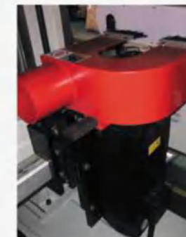
立轴系统(变频马达) H.F Moulding unit 7.5HP (special 10HP 15HP) Spindle speed: 3000/6000 rpm (60/120 HZ) Spindle size: Ø40 x 120 MM (L) Option attachment: Jumping device
