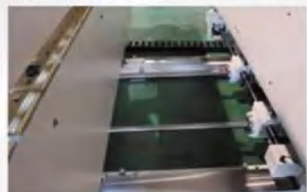
分离式线轨 採用分离式双基座配合滚珠导 螺杆传动 individual linear guide way Two slide guide way transfer with ball screw.
