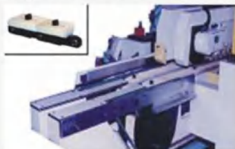
进给链条装置 配备精密履带链条，此履带链条 装置採防尘及免润滑之针状轴承 (厂牌:德国INA) Feed chain track system Is enriched with precision track linkage mounted with dust-proof and free lubricated needle bearing, to ensure perfect parallel at y-axis. (BRAND: GERMAN INA)
