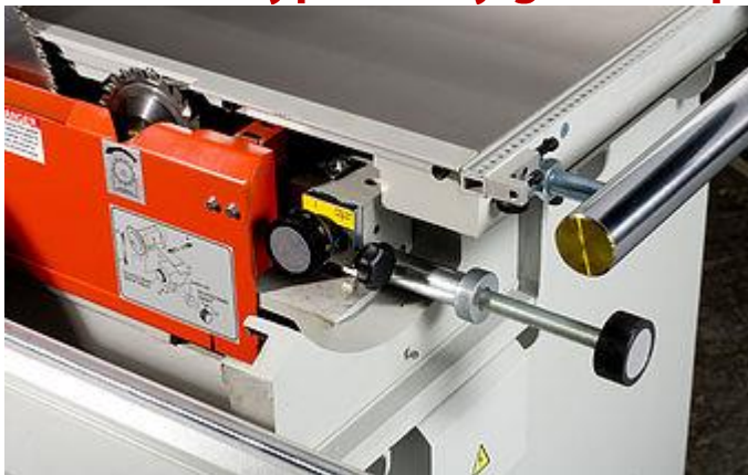
修邊鋸調整 Scoring Blade Adjusting
