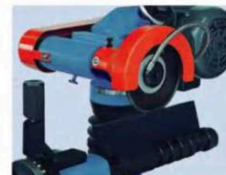
鎢鋼平鉋刀研磨範例 (附件如圖) Typical Applications of Grinding Straight Carbide Knife (Optional accessories shown as fig.)
