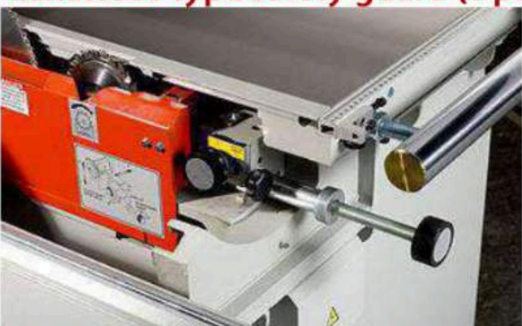
修邊鋸調整 Scoring Blade Adjusting
