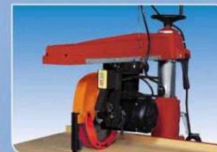
3. Cut with saw blade perpendicular and square to the fence; cutting off. 3. 鋸片切削，與擋板垂直切斷。
