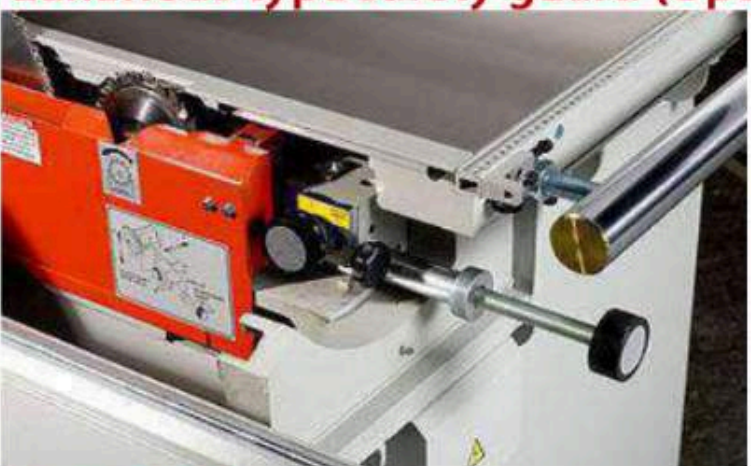
修邊鋸調整 Scoring Blade Adjusting
