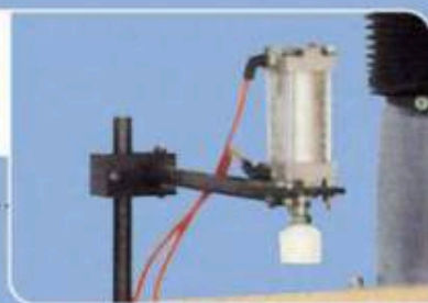
氣壓滾筒式固緊裝置 Pneumatic Cylinder Clamp
