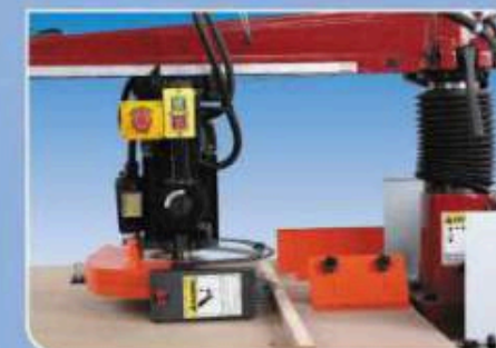
5. Cut or milling with saw blade in horizontal position and parallel to the fence. 5. 鋸片水平位置可切削或銑，與擋板平行。
