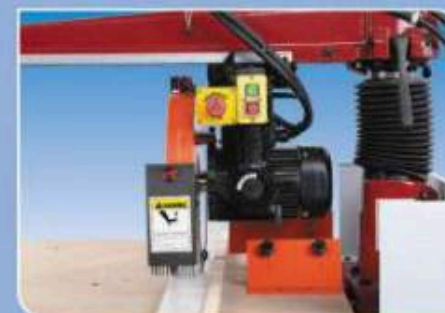
4. Cut with saw blade parallel to the fence for squaring and trimming operations. 4. 鋸片切削，與擋板平行，削直及修整。
