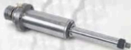
高轉速主軸 (8000 RPM)
