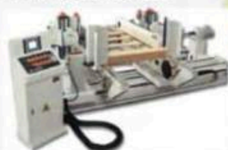
自动送料架 Auto. feeding magazine Working length: 220~1300/2000/2600 mm Working width: 50~150 mm Working height: 8~60 mm Max. working height of magazine: 500 mm
