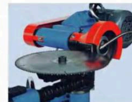
鎢鋼圓鋸片研磨範例 (附件如圖) Typical Applications of Grinding Circular Sawblade (Optional accessories shown as fig.)
