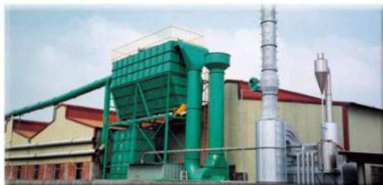
濾管式集塵機 FILTER TYPE DUST COLLECTOR
